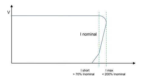
The load characteristic is designed to accomplish reliable start-up of devices requiring full current at reduced output DC voltage. The maximum current will not exceed 200% of the nominal or 8A, whilst the output power will always be less than 100W for normal and overload operation with nominal output voltages (except TBLC 90-112).
