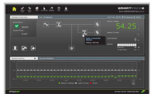
STATUS OF DC/DC CONVERTERS IN SMARTPACK2 WEB
